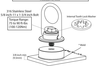
\* Welding procedure must be approved by an engineer or other qualified person to be compatible with any and all structural & operational characteristics of the selected installation location.
