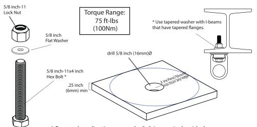
\* For steel applications, a grade-5, 8 (or equivalent) bolt no shorter than 4 inches (100mm) with a locking nut and washer must be used. Swivel anchor must be flush with steel surface. A 16mm bolt may be used in place of a 5/8 inch-11 for metric applications.
