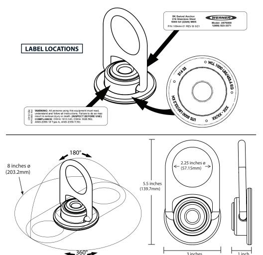
Minimum Breaking Strength (MBS): 5,000-lbf (22kN)
