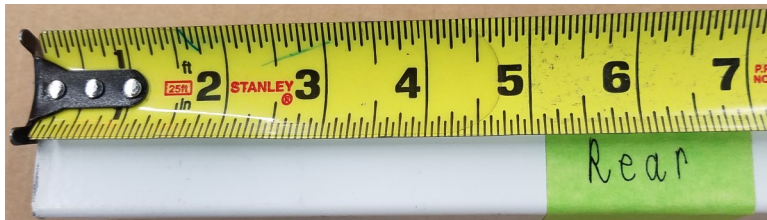
Proper taping of a rear Crossmember for directly mounting on a Ford Transit Connect (5-1/8")
