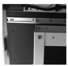
**STEP 17.** Make sure all shelves are aligned and make sure all bolts and nuts are properly torqued to spec. use 76 in-lbs for 1/4-20 hardware and 13 ft-lbs for 5/16-18 hardware.
