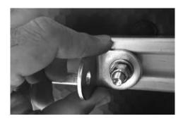
STEP 16. Install the end strap to the L-bracket using 1/4-20 x 3/4" bolt, washer, and nylon lock nut using 7/16" wrench and socket. Position the strap such that it is inline with the end panel. Align the end strap to one of the holes on the end panel and secure it using 1/4-20 x 3/4" bolt, washer, and nylon lock nut. Make sure all components are aligned and tighten.
