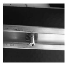
**STEP 11.** Position the shelves and carriage bolts/plates in desired location and fasten the shelves to the carriage bolt/plate using 5/16-18 nylon lock nuts and washers using 1/2" socket. Fine tune the position and alignment of the shelves in desired location. Torque them down to 13 ft-lbs.
