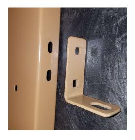
ATTACH THE DOOR LATCH: AS SHOWN USING TWO ¼-20 CARRIAGE BOLTS AND TWO ¼ WHIZ NUTS. HAND TIGHTEN AT THIS POINT.
