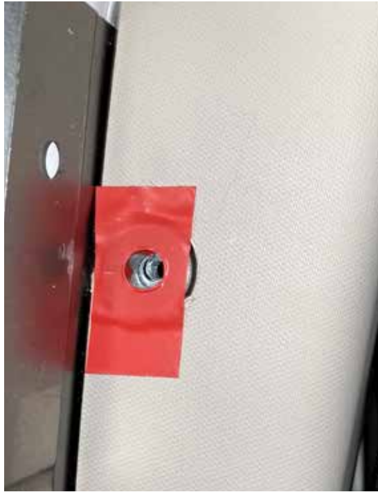
Step 7 Tape Spacers to B-Pillar Trim
