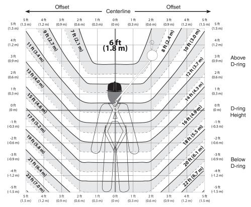
**Example:** Pictured above, with the SRL-LE anchored 4 feet above the users D-ring and the user works 2 feet away (offset) from directly overhead (centerline), the required clearance is 7 feet (2.1m), indicated by the shaded zone in the chart. 7 feet from the working level to the nearest obstruction below is the clearance required for this application.
