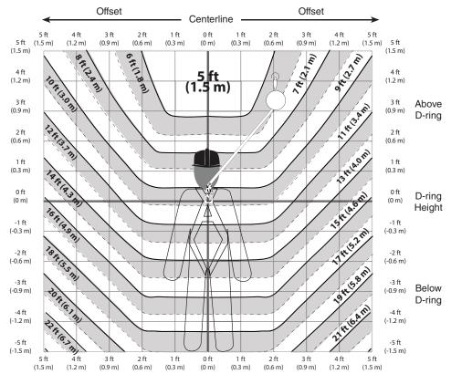
**Example:** Pictured above, with the SRL-LE anchored 4 feet above the users D-ring and the user works 2 feet away (offset) from directly overhead (centerline), the required clearance is 6 feet (1.8m), indicated by the shaded zone in the chart. 6 feet from the working level to the nearest obstruction below is the clearance required for this application.
