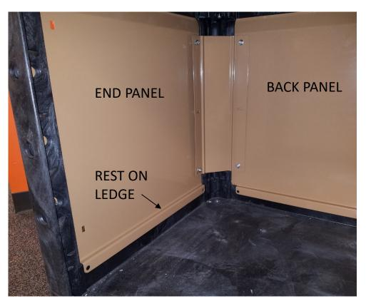
END PANEL INSTALL: ON A SHORT SIDE OF THE CART, LET THE BOTTOM OF THE END PANEL REST ON THE LEDGE OF THE CART. ATTACH TO PREVIOUSLY INSTALLED CORNER CLAMP USING TWO CARRIAGE BOLTS AND TWO ¼-20 WHIZ NUTS. HAND TIGHTEN AT THIS POINT.
