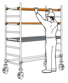
**3** Fit two diagonal braces (blue) in opposing directions between the 2nd and 6th rungs. Ensure the frames are vertical and level by checking with a spirit level and setting the adjustable legs as necessary. Fit the next pair of end frames and check the frame interlock clips are engaged. Fit stabilisers (see notes on page 30).
