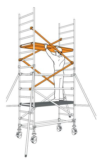
**5** Climb up the inside of the tower and from the protected position of the trapdoor, fit horizontal braces as guardrails (on both sides) to the 14th and 16th rungs (2 and 4 rungs above the platform in that order).
