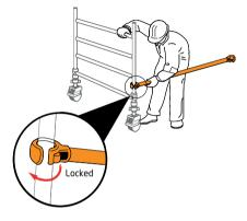
**3** Position the second end frame as shown and at the other end of the horizontal brace onto the vertical, just above the bottom rung. Fit a second horizontal brace between the bottom rungs on the other side of the frames to square the tower.
