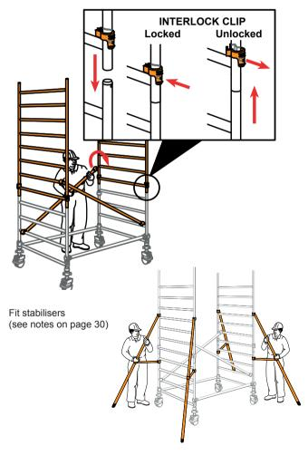
**5** Fit a temporary deck on the lowest rungs. Fit a trapdoor deck on the 8th rung (2.0m) on one side of the tower. Ensure that the trapdoor is positioned with the hinges towards the outside of the tower as shown. Climb the end frame below the trapdoor on the inside of the tower, and from within the protected trapdoor position, fit horizontal braces on the 10th and 12th rungs (in that order) on both sides of the deck.
