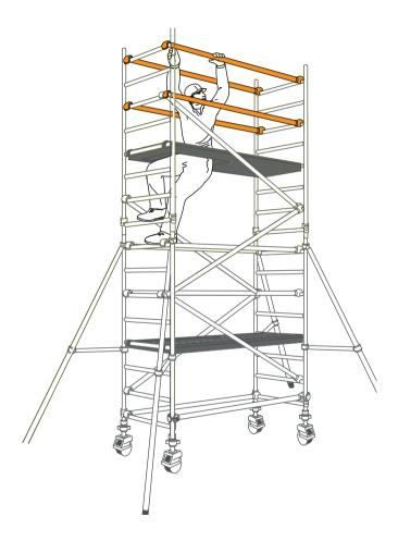
Continue the procedure until the required working height is reached, adding additional pairs of end frames, diagonal braces and fitting trapdoor platforms, as shown on previous steps. At every platform level, add horizontal braces as guardrails at 2 and 4 rungs above the platform (in that order) on both sides of the platform. (as shown in Step 5).
