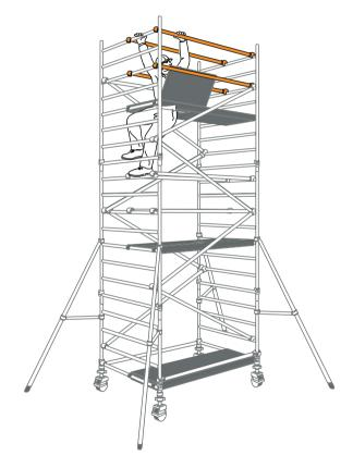
Continue until the required height is reached. Re-position the fixed deck to the required platform height and fit a trapdoor deck alongside it as shown in Stage 7. Fit the guardrails as shown in Stage 7.
