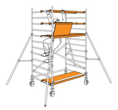
**6** Fit the next pair of diagonal braces in opposing directions between the 6th and 10th rungs add two additional end frames.
