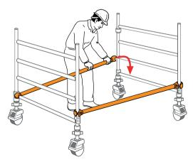
Fit two additional end frames and check that the frame interlock clips are engaged. Fit two diagonal braces (blue) in opposing directions between the 2nd and the 6th rungs. Ensure the frames are vertical and level by checking with a spirit level and setting the adjustable legs as required.
