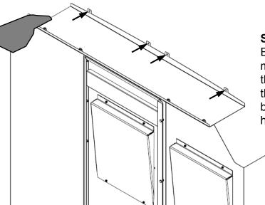
STEP 7. With the Bulkhead against the B-Pillar trim, use a marker or pencil and mark the four Bulkhead header holes on the roof panel. Move the Bulkhead out of the way. Drill a pilot hole with an 1/8" drill bit. Cut the roof trim with a knife or 1" hole saw if necessary.
