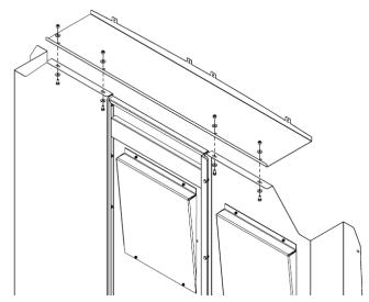
**STEP 4.** Attach the Header Support (Same panel for either Standard or High Roof vans). to the Bulkhead using four (4) 1/4-20 x 5/8" Hex Head Bolts, eight (8) 1/4" Flat Washers and four (4) 1/4-20 Nylon Lock Nuts.
