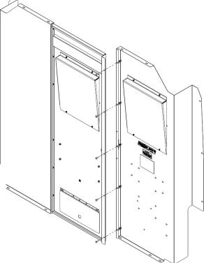
**STEP 3.** Attach Passenger Side Panel to Center Panel with both panels flush to the bottom using five (5) ½-20 x 5/8" hex head bolts, ½" flat washers, and ½-20 lock nuts.
