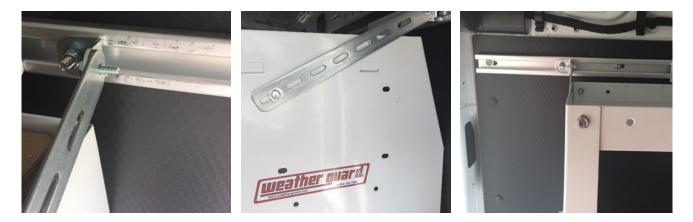
**STEP 16.** Make sure all shelves are aligned and make sure all bolts and nuts are properly torqued to spec. use 76 in-lbs for 1/4-20 hardware and 13 ft-lbs for 5/16-18 hardware.
