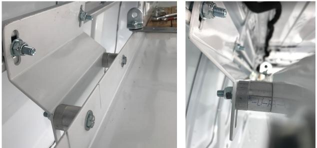
**STEP 8.** Position the carriage bolt plate such that you can read the word "TOP" and insert 5/16-18 carriage bolt from the bottom of the plate. Note: using a piece of masking tape (or equivalent) on back of the plate to lightly hold the carriage bolt to the plate may allow easier installation. You will need four plates per shelving unit plus two for each side (driver/passenger) for the end straps.
