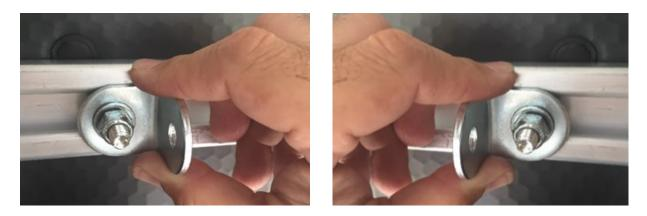
**STEP 15.** Install the end strap to the L-bracket using 1/4-20 x 3/4" bolt, washer, and nylon lock nut using 7/16" wrench and socket. Position the strap such that it is inline with the end panel. Align the end strap to one of the holes on the end panel and secure it using 1/4-20 x 3/4" bolt, washer, and nylon lock nut. Make sure all components are aligned and tighten.
