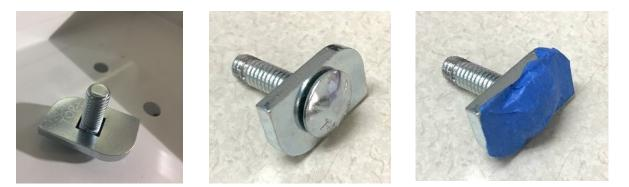
**STEP 9.** Insert the carriage bolt/plate assemblies through the mounting channel and rotate 90 degrees clockwise. Ten will be used on driver side and six will be used on passenger side when installing standard configuration of two and one shelving for driver side and passenger side, respectively. Note: 148" EXT Vans use three shelves on the driver side, thus, will require 14 carriage bolts/plates on driver side.
