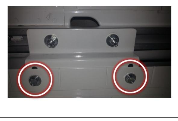
**STEP 14.** Loosely assemble L-bracket for the end straps to the carriage bolt/plate assembled in **STEP 8.** L-brackets and end straps are included with the shelf. Use washer and 5/16-18 nylon lock nut using 1/2" socket. The face of the L-bracket that is perpendicular to the mounting channel may face front or rear of the van depending on the shelf size and configuration.
