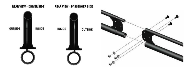
STEP 4 Install the rear leg, with the tie down facing the outside using (1) Part C, (1) Part L, and (1) Part F.
