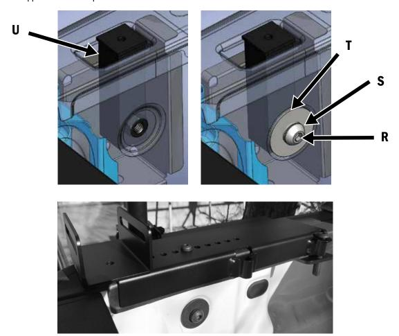
**STEP 16** Measure the distance from center to center of mounting foot bed and set the rack assembly accordingly. Tighten all hardware with a 3/8"-16 button head to a 15 ft-lb torque and tighten all other hardware to a 25 ft-lb torque except the front legs hardware. (DO NOT TIGHTEN THE SET SCREWS ON THE FRONT LEGS).
