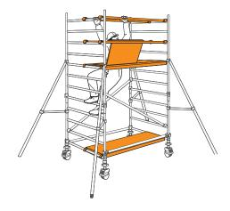
Fit the next pair of diagonal braces in opposing directions between the 6th and 10th rungs add two additional end frames
