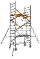
Continue the procedure until the required working height is reached, adding additional pairs of end frames, diagonal braces and fitting trapdoor platforms, as shown on previous steps. At every platform level, add horizontal braces as guardrails at 2 and 4 rungs above the platform (in that order) on both sides of the platform (as shown in Step 5).
