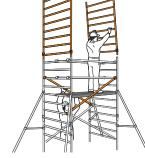
Add two more diagonal braces between the 10th and 14th rungs. If finishing at this height (4.2m platform), the fixed deck should be repositioned to the 16th rung on the opposite side of the tower to the trapdoor deck. Fit a trapdoor deck alongside it with the hinges towards the outside of the tower and the trapdoor in line with the one below. Climb the tower and from the protected trapdoor position, fit the horizontal braces as
