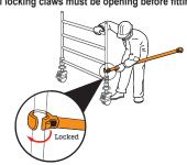
Position the second end frame as shown and at the other end of the horizontal brace onto the vertical, just above the bottom rung. Fit a second horizontal brace between the bottom rungs on the other side of the frames to square the tower.
