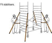
Fit a temporary deck on the lowest rungs. Fit a trapdoor deck on the 8th rung (2.0m) on one side of the tower. Ensure that the trapdoor is positioned with the hinges towards the outside of the tower as shown. Climb the end frame below the trapdoor on the inside of the tower, and from within the protected trapdoor position, fit horizontal braces on the 10th and 12th rungs (in that order) on both sides of the deck.
