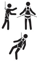
This harness is equipped with Gravity Override. In the event of a Fall, grab the relief handles and pull out and forward, while lifting legs to a seated position. See user instructions for more information.
