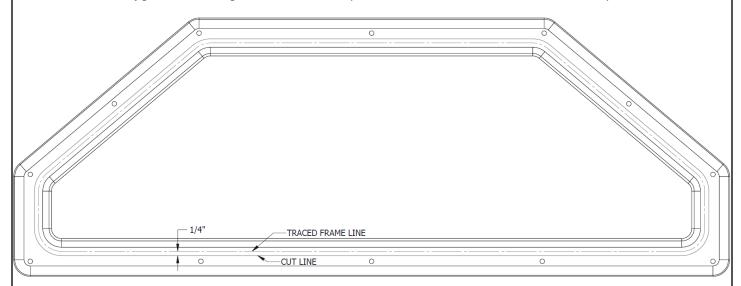
STEP 7 Use #10-24 screws, washers, and nylon lock nuts to attach the window panel and frames to the bulkhead panel. The window panel will sit within the recess (on the cargo side) of the bulkhead with a frame on the outside of the window panel sandwiching it against the bulkhead. The other frame will be on the embossed/cab side of the bulkhead. Tighten to 23 in-lbs.
