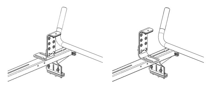
**NOTE:** Use option 1 for most standard extension ladder applications and option 2 for dead-head ladders and some step ladder applications.
