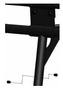
**STEP 16** Measure the distance from center to center of mounting foot bed and set the rack assembly accordingly. Tighten all hardware with a 3/8"-16 button head to a 15 ft-lb torque and tighten all other hardware to a 25 ft-lb torque except the front legs hardware. (DO NOT TIGHTEN THE SET SCREWS ON THE FRONT LEGS).
