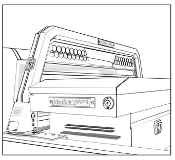
Align the adhesive tape to the leveling spacer to the truck box, slightly inset from side.
