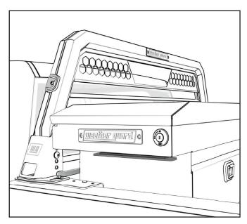
Make sure the bottom corner surface is free of debris or liquid to insure proper adhesion of the double sided fastener. Mount the tape and leveling spacer to the truck box.
