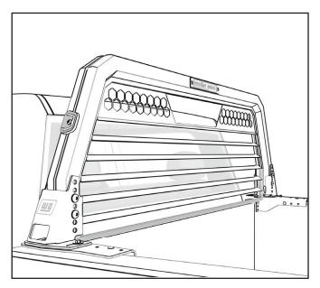
Prior to installation of the leveling spacer the headache rack must be installed.
