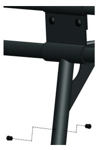
**STEP 16** Measure the distance from center to center of mounting foot bed and set the rack assembly accordingly. Tighten all hardware with a 3/8"-16 button head to a 15 ft-lb torque and tighten all other hardware to a 25 ft-lb torque except the front legs hardware. (DO NOT TIGHTEN THE SET SCREWS ON THE FRONT LEGS).
