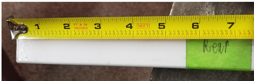
Proper taping of a rear Crossmember (5-5/8")
