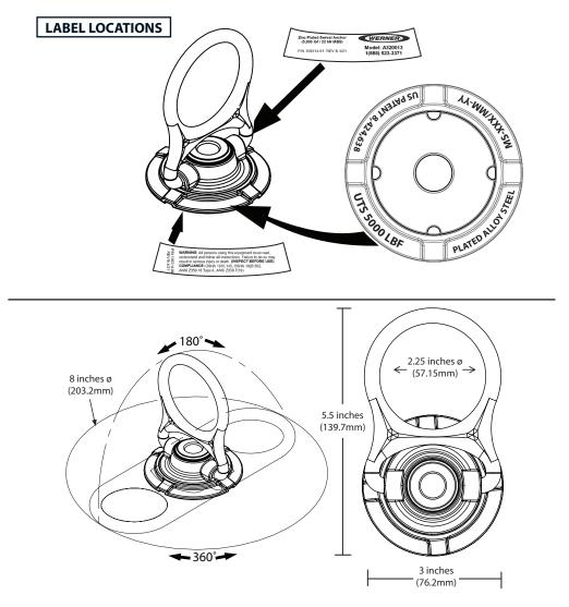
Tensile Strength (UTS): 5,000-lbf (22kN) Weight: 1.2-lbs (544.3g) Materials: Zinc Plated Steel Regulatory Compliance: Meets or exceeds ANSI Z359.18 Type A, ANSI Z359.7-2019 OSHA 29 CFR 1926.502, OSHA 29 CFR 1910.140
